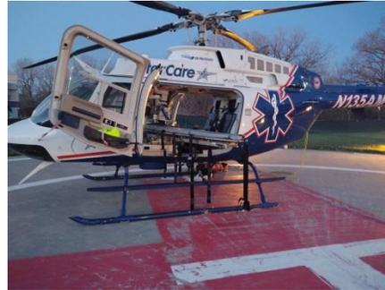
**SIDE-LOAD CONFIGURATION WITH SLED STRETCHER.**
